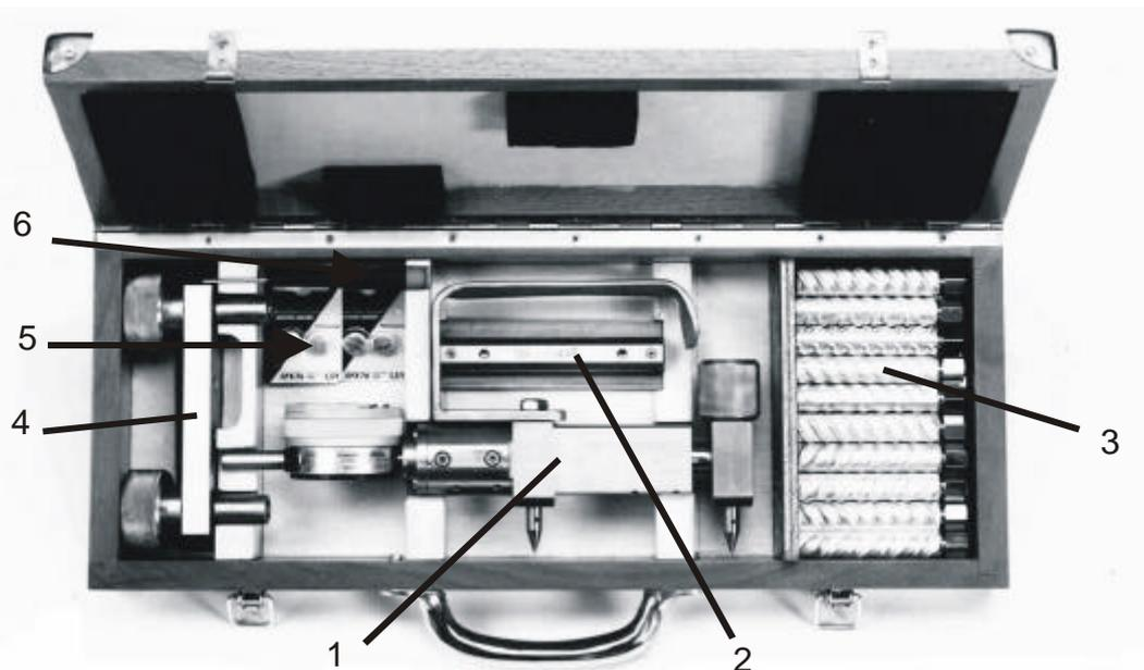
Fig. 1 Mechanical fissurometer type FM 100 with accessories. 1 Fissurometer, 2 Calibration device made of INVAR steel, 3 Measuring rod type FB 70, 4 Setting gauge, 5 Spare batteries for electric dial gauge, 6 Screwdriver for changing the battery
