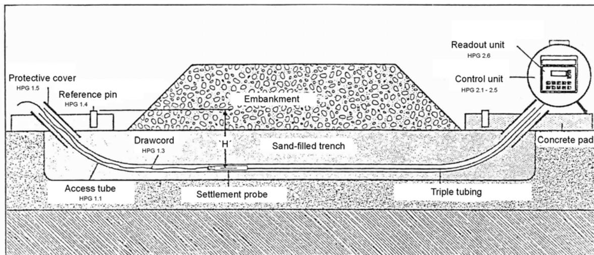
Fig. 1 Schematic arrangement of a measuring setup for levelling with a mobile hydrostatic profile gauge
