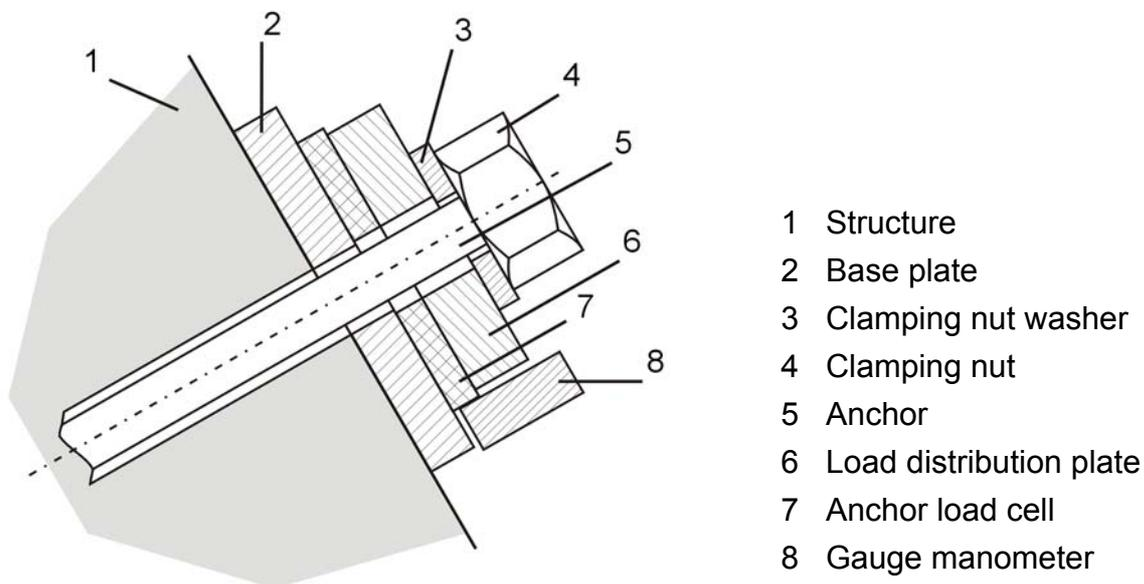
Fig. 2 Head configuration of a rock anchor with a direct-reading anchor load cell Type M
