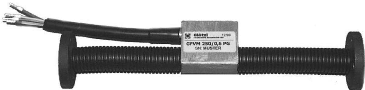
Fig. 1 Measuring sensor GFVM 250/0.5 for concrete strain measurements, based on the vibrating wire measurement process
