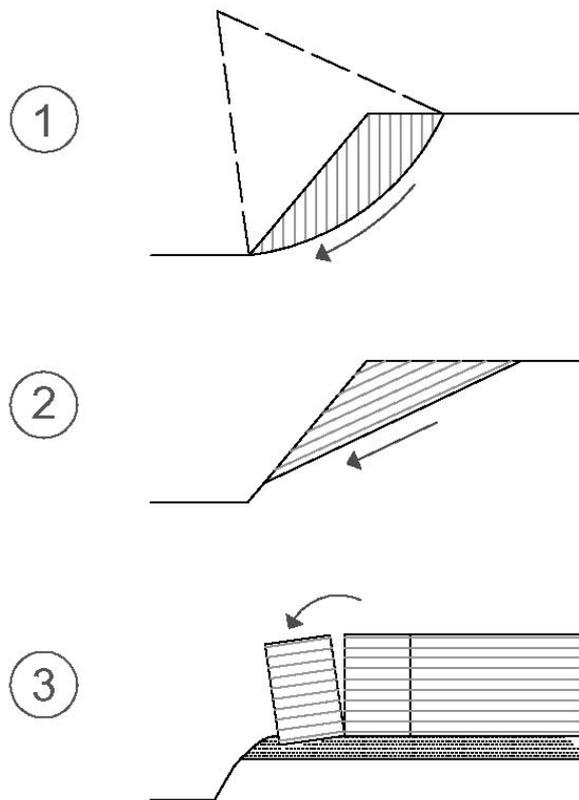
Fig. 1 Different movement mechanisms in the development of slope slides
