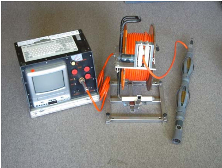
Fig. 1 Components of the borehole video inspection probe
