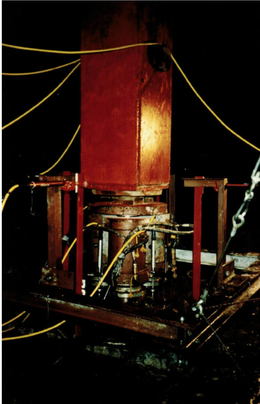
Fig. 4 Triaxial test in the access gallery of the cavern Cirata, Indonesia
