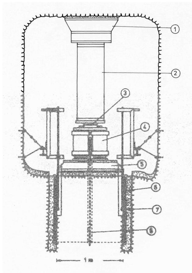
Fig. 1 In situ triaxial test on a specimen of 1 x 1 x 1 m
