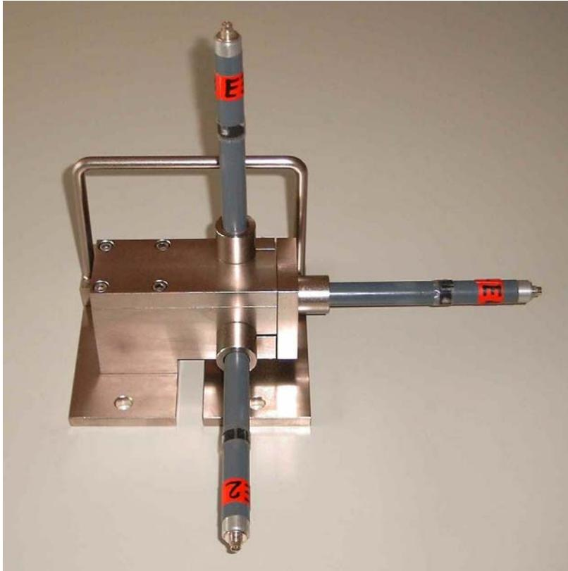
Fig. 2 Setting device type F3E with electrical reading
