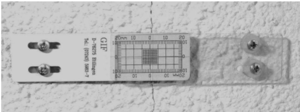
Fig. 1 Crack spy in its standard version
