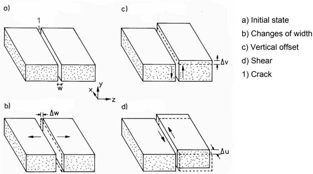
Fig. 1 Possible displacements of crack flanks and their coordinates
