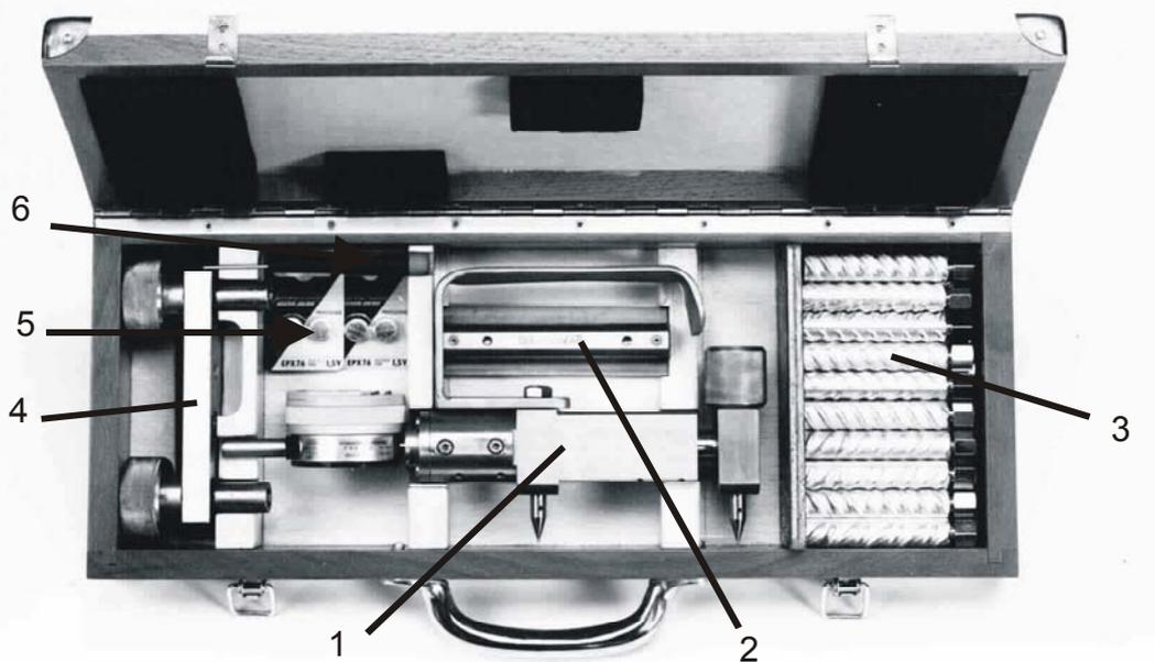
Fig. 1 Mechanical fissurometer type FM 100 with accessories. 1 Fissurometer, 2 Measuring rod type FB 70, 3 Calibration device made of INVAR steel, 4 Setting gauge, 5 Spare batteries for electric dial gauge, 6 Screwdriver for changing the battery
