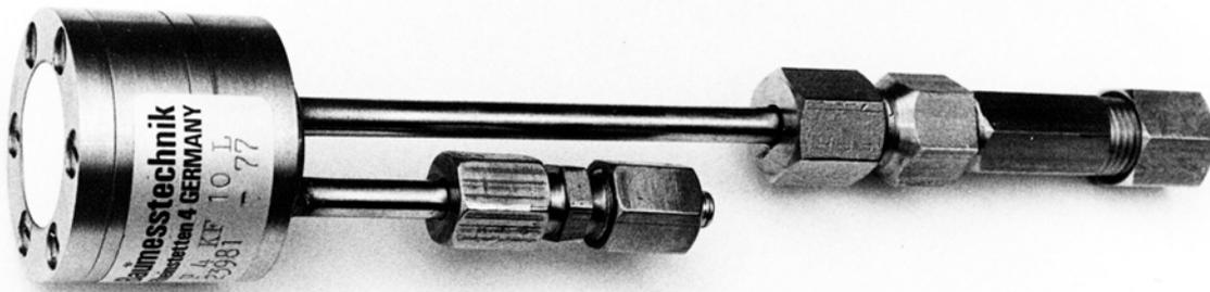
Fig. 2 Porewater pressure transducer Type P 4, KF, 10 L, for installation in a borehole and pneumatic measurements up to a maximum of 10 bar
