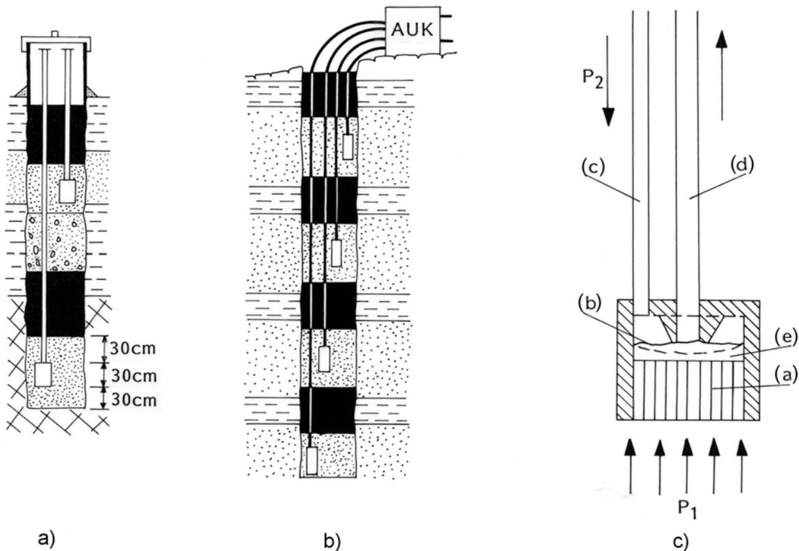
Fig 2 Measurement of water pressures in various aquifers
