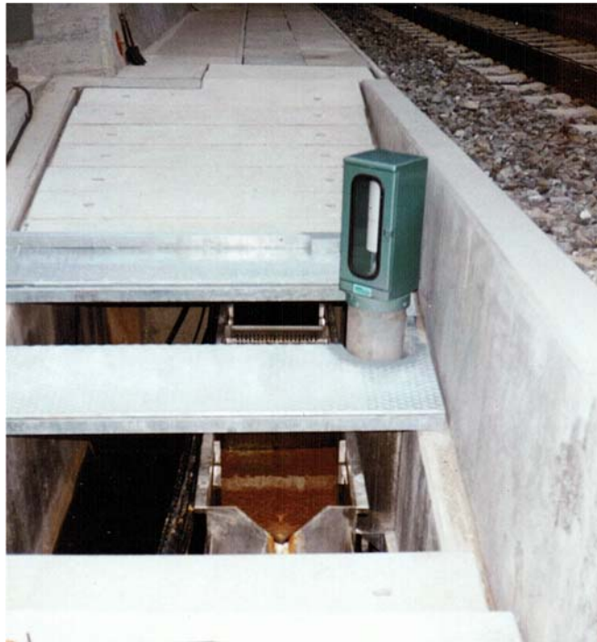
Fig. 2 Measuring weir (3 m long) with a THOMSON triangular overflow and a level logger
