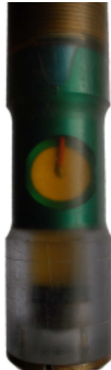
Fig. 1 Rotating ultrasonic transducer of the borehole scanner in oil bath
