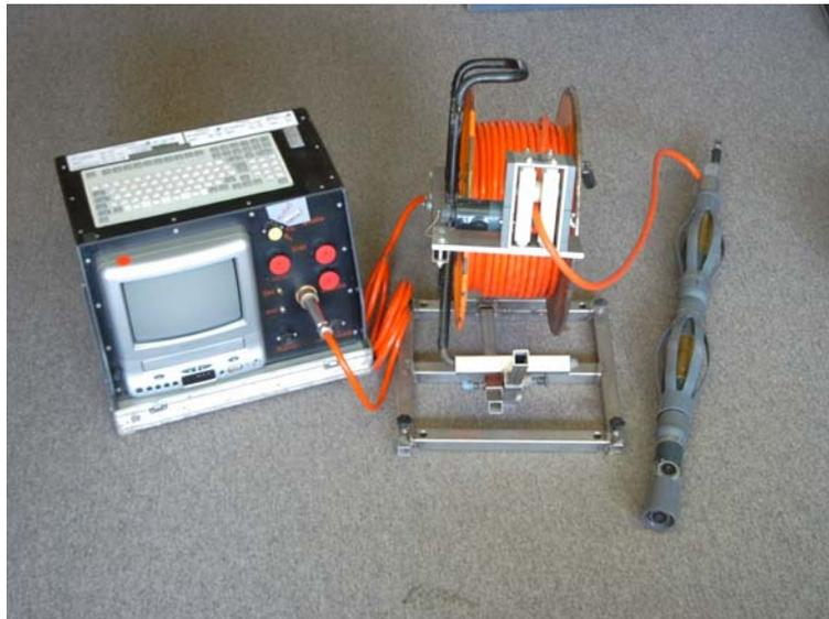
Fig. 1 Components of the borehole video inspection probe
