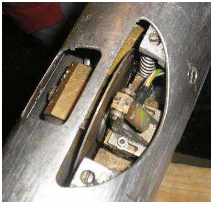
Fig. 2 Strain sensor besides the diamond saw blade
