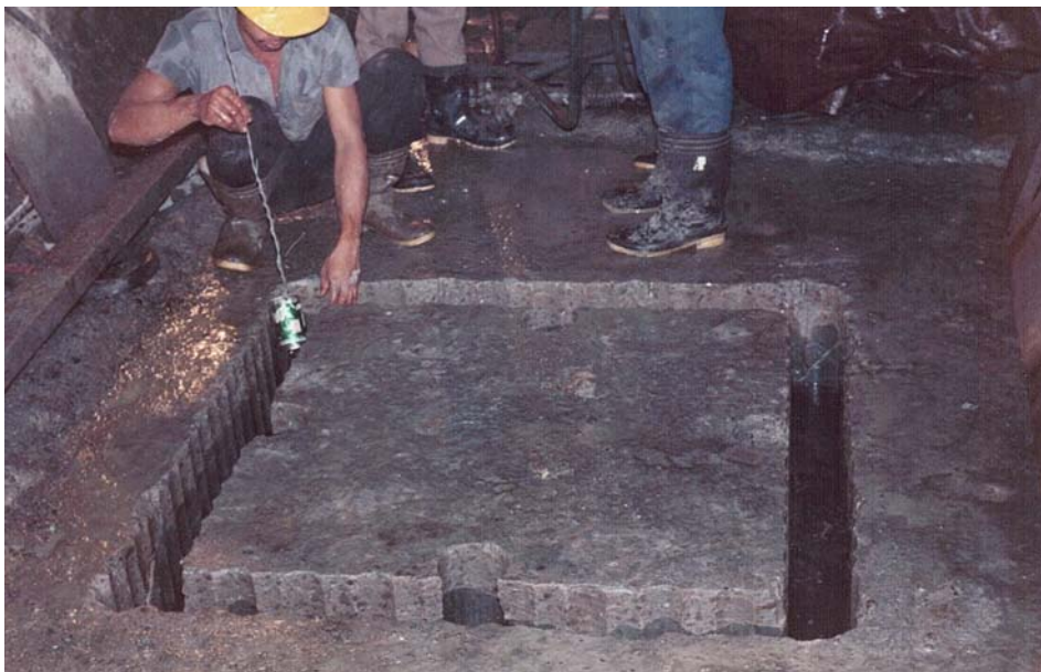
Fig. 3 Slotting the specimen by boring hole to hole
