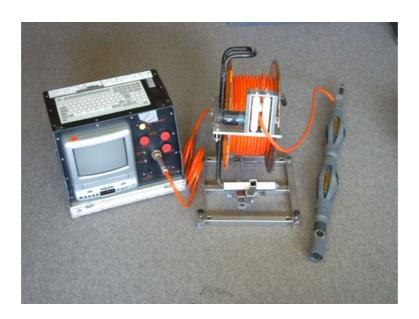
Fig. 1 Components of the borehole video inspection probe
