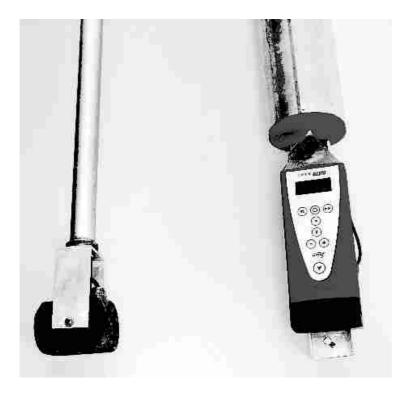
Fig. 1 Acoustic log sensor (left) and laser sensor (right)
